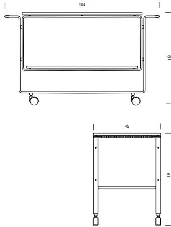
**Materials** Bar Cart with handgrip in leather and two black trays with oakedges. Frame in chrome-plated steel.
